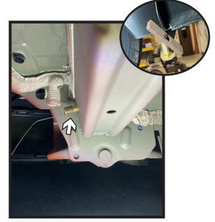
Place spacer plate onto wire then attach lead wire to the end of the 1/2" carriage bolt (inset). Pull bolt and spacer plate through the frame. Repeat process with second bolt hole. Ensure spacer plates are sitting flush against inner frame and the bolts are hanging vertically. Do this on both sides of the vehicle.
