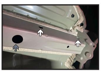
Starting with the rear hole, feed lead wires from holes in the side of the frame (white) to the large access hole (gray) or rear frame hole if available. Do this on both sides of the vehicle.
