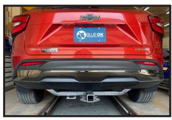
3. Raise hitch into position. Remove lead wires and loosely install 1/2" whiz flange nut onto each bolt. Then tighten all bolts.
